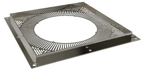
**EN Ventilated firestop plate.** This component is used where the chimney passes through a combustible floor or ceiling. This plate gives the required 50 mm distance from the external part of the chimney to combustible materials. The slots let a suitable ventilation to avoid heat accumulation inside the framing or the enclosure of the chimney.
